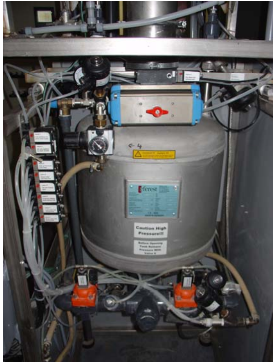
Figure 2. Feed mixing tank of the liquid feeding system at the University of Guelph.
