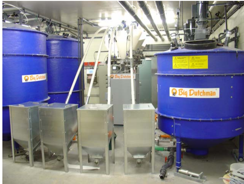
Figure 1. Overview of feed kitchen of the liquid feeding system at the University of Guelph.
