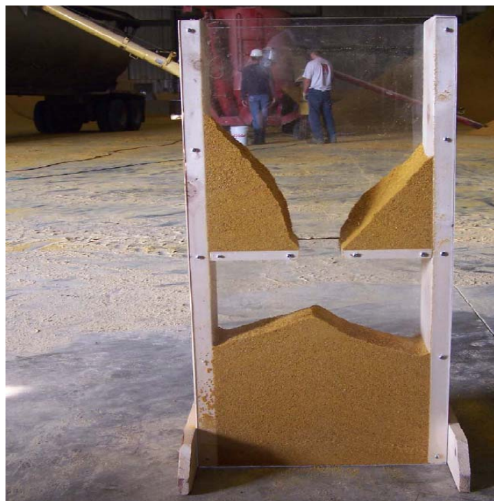
Figure 4. Equipment for measuring Angle of Repose. (Shurson, 2007)
